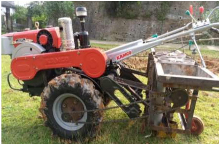
Fig 3. Ginger planter hitched with a power tiller
